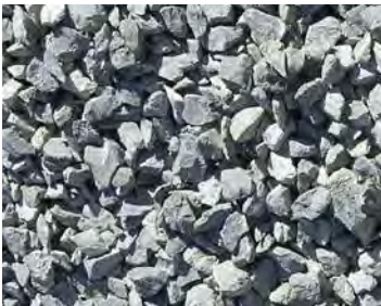
1 1/2 Inch Crushed stone
