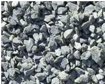
1 1/2 Inch Crushed stone
