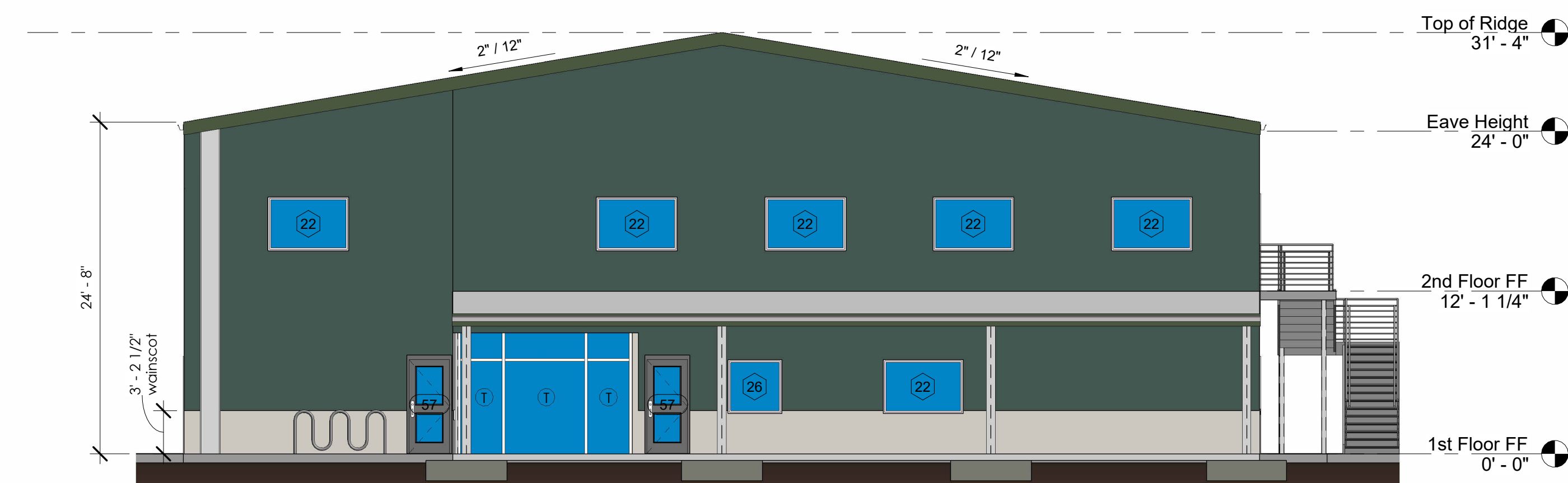
3 Building #2 West Elevation A6.1 1/8" = 1'-0"
