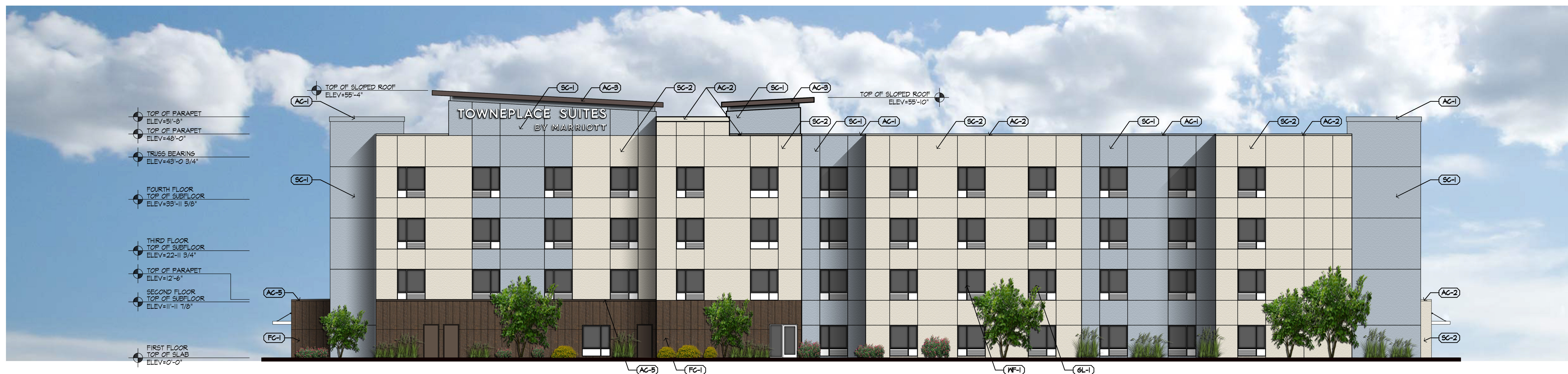
2 A2.1 EXTERIOR ELEVATION @ REAR 3/32"=1'-0"
