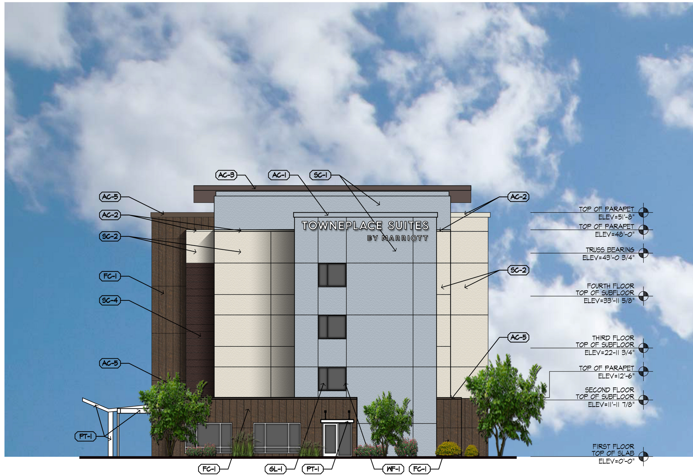
1 EXTERIOR ELEVATION @ SIDE A2.2 3/32"=1'-0"
