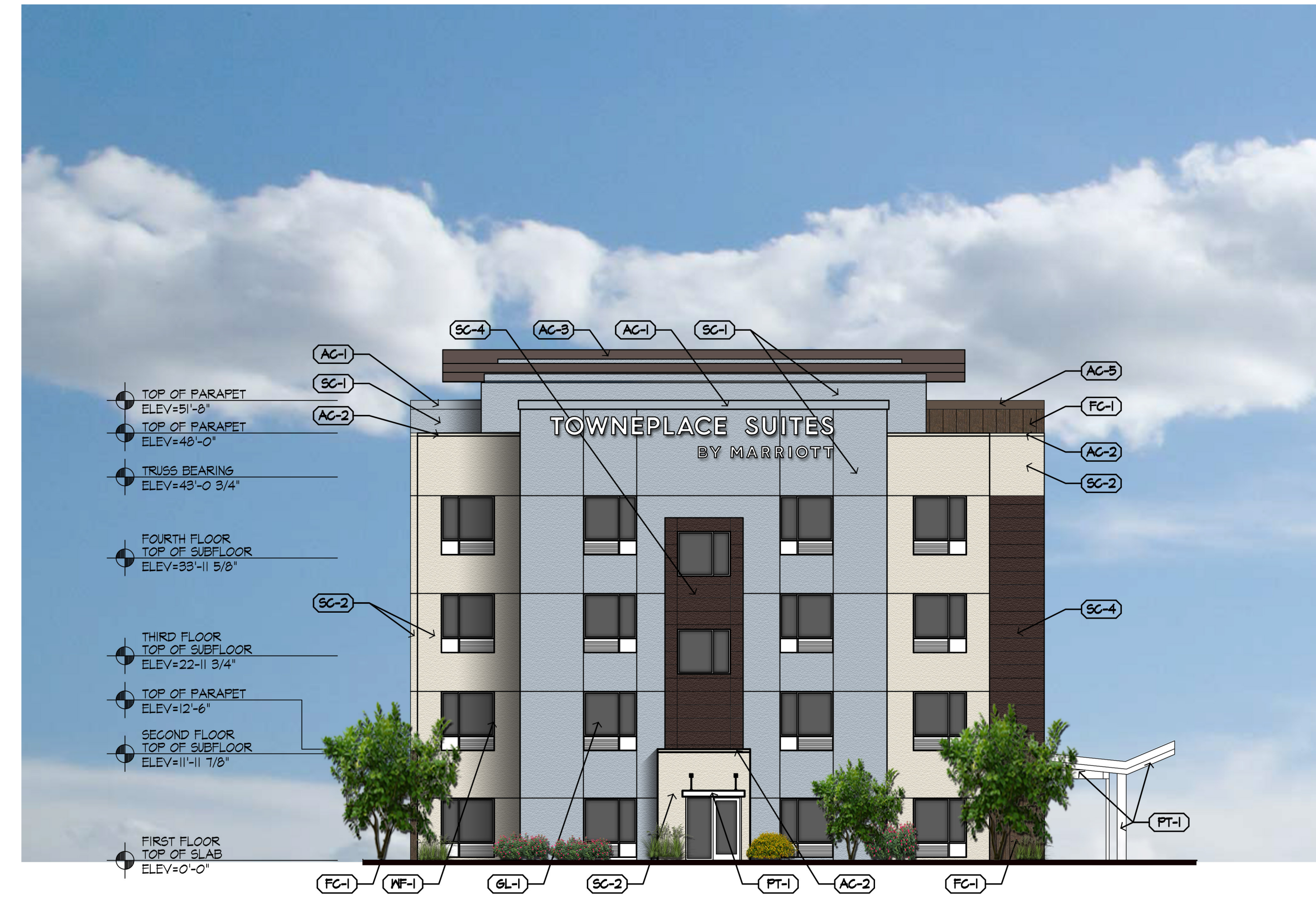
2 EXTERIOR ELEVATION @ SIDE A2.2 3/32"=1'-0"
