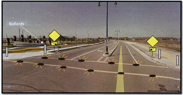
Option 3: In-roadway lights, signage, automatic pedestrian detection and overhead warning lights
