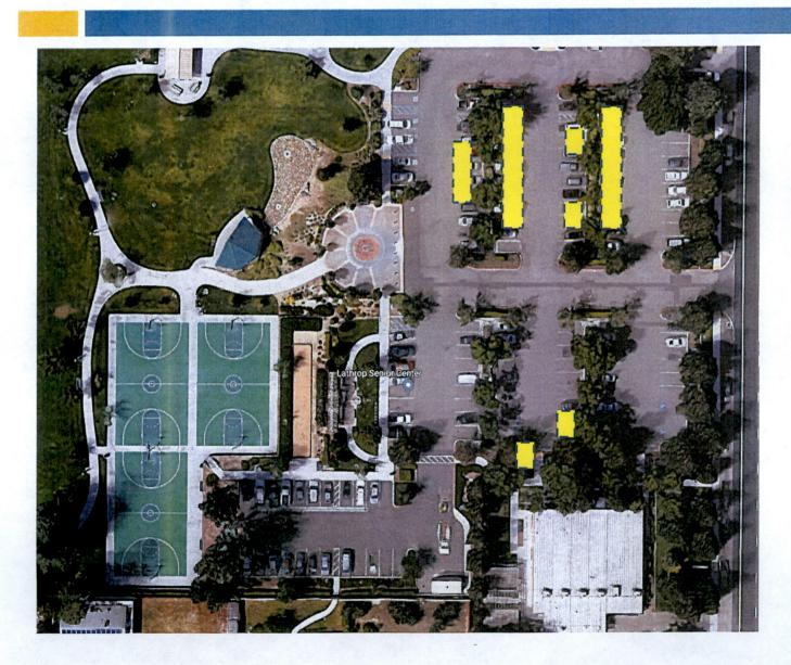
The Asphalt, curb, and gutters will be removed in areas as indicated.
