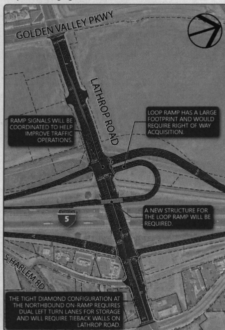
1. TIGHT DIAMOND AND PARTIAL CLOVERLEAF This alternative would widen Lathrop Road under I-5, widen northbound ramps, construct a new loop ramp and diagonal on/off-ramps. The benefit to this alternative is the efficient signal operations at the southbound ramps, better lane utilization on Lathrop Road, and increased spacing between ramp traffic signals.
